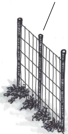
Chicken wire or hardware cloth supported by rebar
