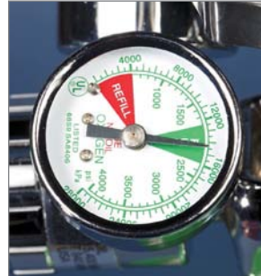
Figure 8-15 | A pressure regulator is attached to an oxygen cylinder to reduce the pressure of oxygen to a safe level.
