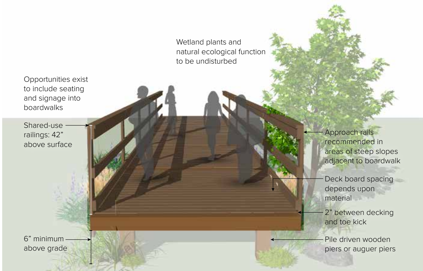
FIGURE 4G Typical bridge/boardwalk cross-section.
