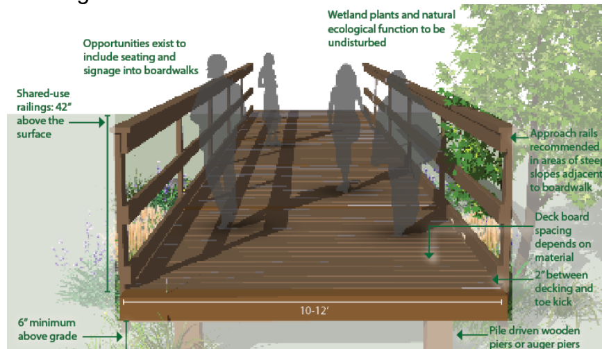
Figure 4G – Typical bridge/boardwalk cross-section.
